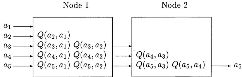
Figure 6: Precedence matrix of a pipeline.
